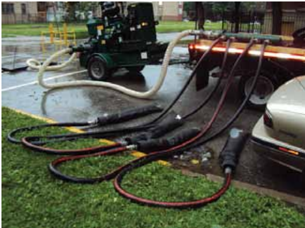
Multiple EVACs can be used with larger pumps with a multi-port manifold.
