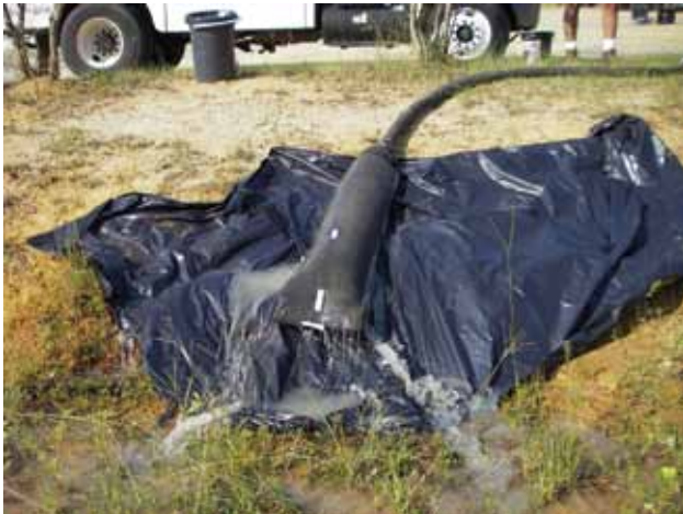
EPA uses EVAC to filter water from frac tank.
