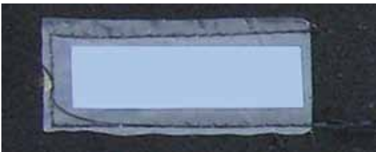
Hydrocarbon Detection Strip placed against outer skin.
