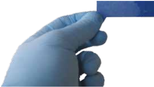
The Hydrocarbon Detection Strip turns a darker blue when hydrocarbons are present.
