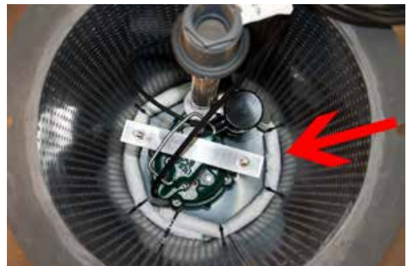
C.I.Agent Quick Deployment Boom lining inside of Filter Strainer and outer bottom of Pre-filter (not shown)
