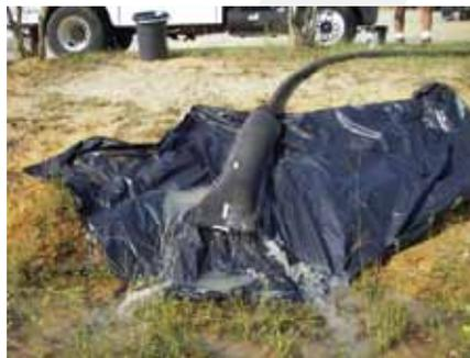
C.I.Agent® EVAC Filter is attached to a hose from the frac tank. The water is filtered to a non-detect level for hydrocarbons.
