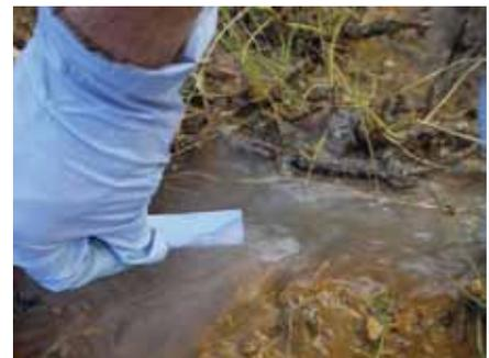
A C.I.Agent® Hydrocarbon Detection Strip is used to monitor the filtered water leaving the EVAC Filter.
